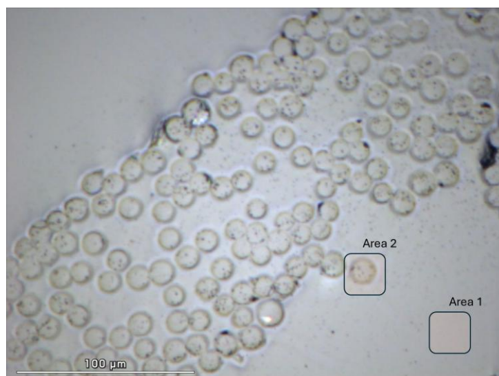
Figure 5. Optical micrograph of the polished cross-section of glass fibers embedded in an epoxy matrix, showing the nanoindentation test locations (Area 1, resin-only region and Area 2, region containing a single glass fiber, scale bar = 100 \mu\text{m} ).
